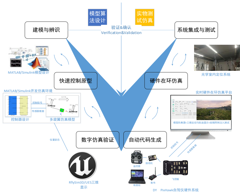
FIG. 1 Model-based design block diagram of RFLySim platform1
