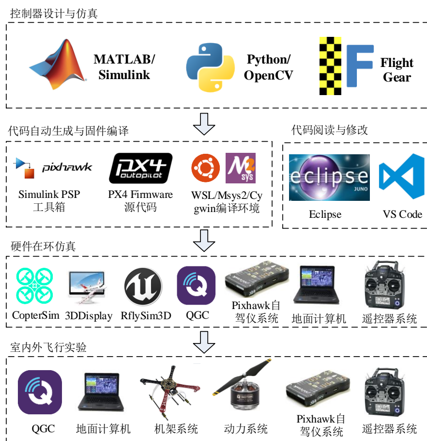
Figure1 Interrelationship between RflySim hardware and software components and the overall process
