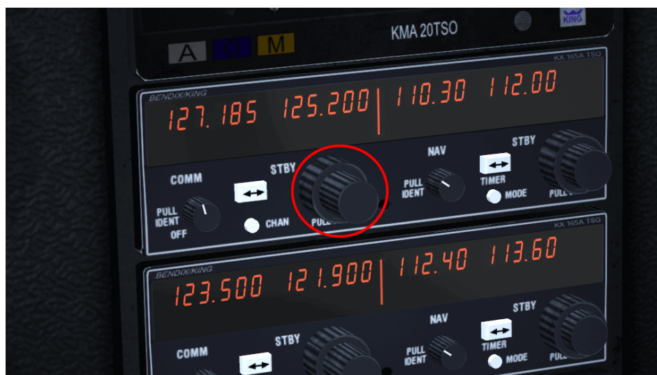
Figure 9.5: COMM1 adjustment knob
