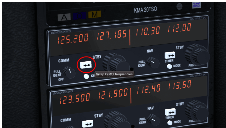
Figure 9.6: COMM1 transfer key to swap the frequencies
