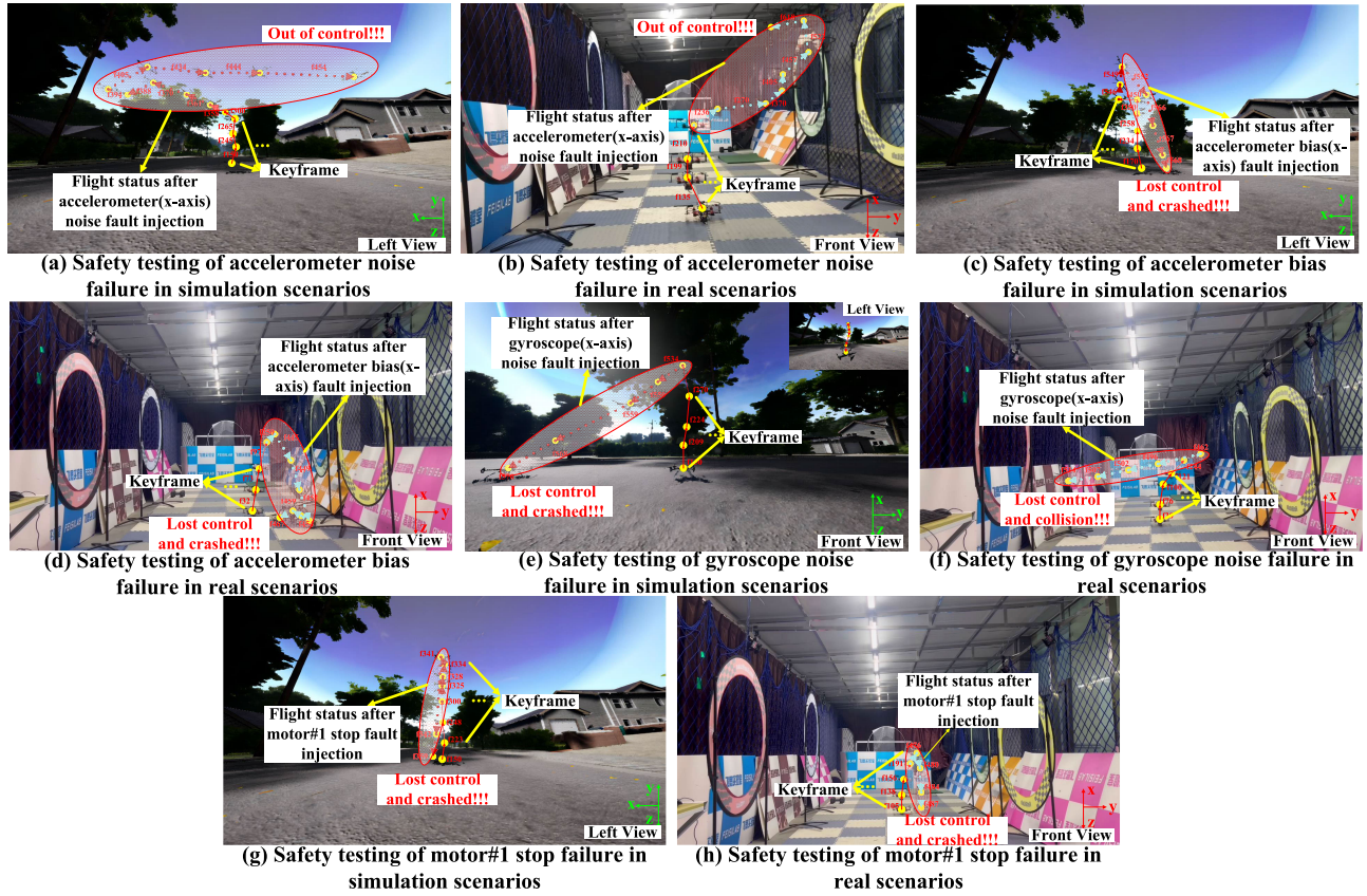
Fig. 11. Keyframe visualization comparisons of HIL simulation and real flight under identical task conditions for four failure modes: accelerometer noise, accelerometer bias, gyroscope noise, and motor failure. Figures (a) and (b) respectively depict the results after injecting accelerometer Gaussian noise faults (mean: 0 \text{ m/s}^2 , variance: 50 \text{ m/s}^2 ) in HIL and real-flight scenarios. Figures (c) and (d) depict the results after injecting accelerometer x-axis bias faults (bias magnitude: 40 \text{ m/s}^2 ) in HIL and real-flight scenarios. Figures (e) and (f) depict the outcomes following the injection of gyroscope Gaussian noise faults (mean: 0 \text{ rad/s} , variance: 5 \text{ rad/s} ) in HIL and real-flight scenarios. Figures (g) and (h) depict the results after injecting motor#1 stop faults in HIL and real-flight scenarios. The yellow segments represent critical frames in the aircraft’s motion, while the circular regions denote the flight states following the injection of faults.
